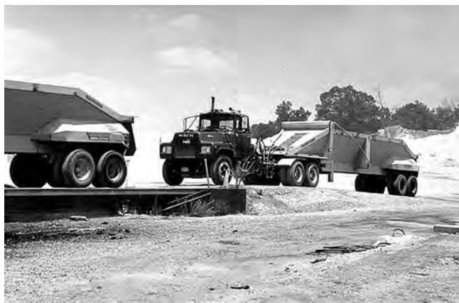
FIGURE 13-4 Typical live-bottom truck.
