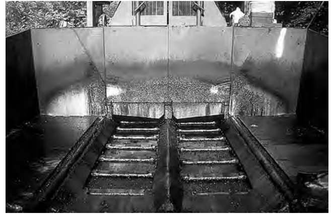
FIGURE 15-5 Slat conveyors at bottom of paver hopper.
