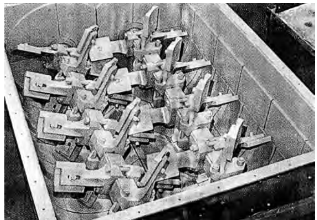
FIGURE 8-4 Interior of pugmill.
